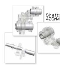
Shafts are made from 42CrMo4 steel and tempered to reach a hardness of 23-35 HRC. thus increasing their capacity to withstand shearing stresses and torsion effect.
