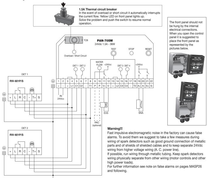
No connection on spark detectors terminal "S".
