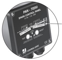
In the packaging are included no 8. "NOT PRESENT" labels to put on the front panel to advise that one or more components are missing.
