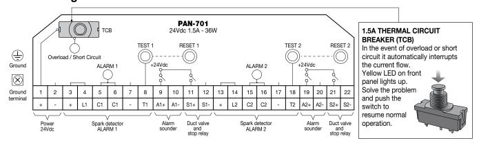
For each line (ALARM 1 and ALARM 2) an additional "C" terminal is available to add another spark detector.
