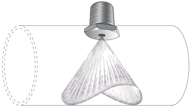
Note: install a pair of nozzles to achieve an effective extinguishing barrier. The two nozzles of the pair are mounted on the sides, horizontally opposite each other.
