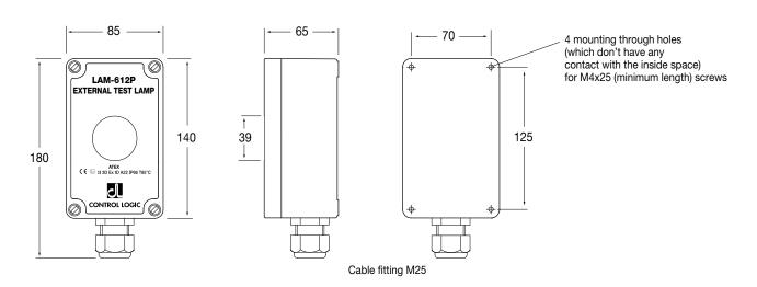
Notes: In order to ensure an <u>IP66 protection grade</u> the cover must be tightly closed turning the four screws provided. The suggested closing torque value is  $1 \div 1.5$ Nm.
