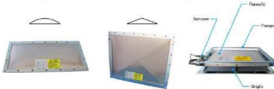
The anti explosion panels at predetermined breaking, certified with the EN14797 norm, are safety devices against the overpressure in the storage's equipments or transport of inflammable materials.
