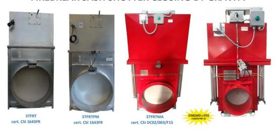
Firebreak sash shutter with closure by gravity have been designed to leave all the passage surface free in the pipe, it's a very important element in the extraction systems where there is material or dust in transit in the air. In the sash shutter the diaphragm is completely outside the passage of the material and it remains intact over time.
