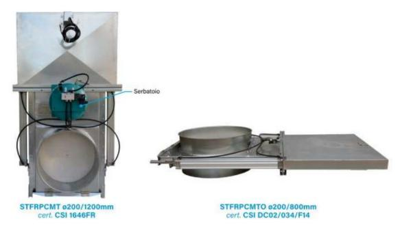
Firebreak sash shutter pneumatic closing have been designed to leave all the passage surface free in the pipe, a very important element in the extraction systems where there is material or dust in transit in the air. In the sash shutter the diaphragm is completely outside the passage of the material and remains intact over time.
